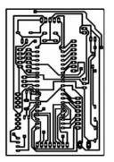
Top and bottom layers of PCB for Receiver part
