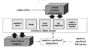
given fully qualified names. Each Java virtual machine also has an execution engine: a mechanism responsible for executing the instructions contained in the methods of loaded classes.
